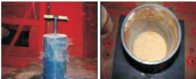
Figure 8 – Vibration test plus 10 kPa (K=9) pressure
