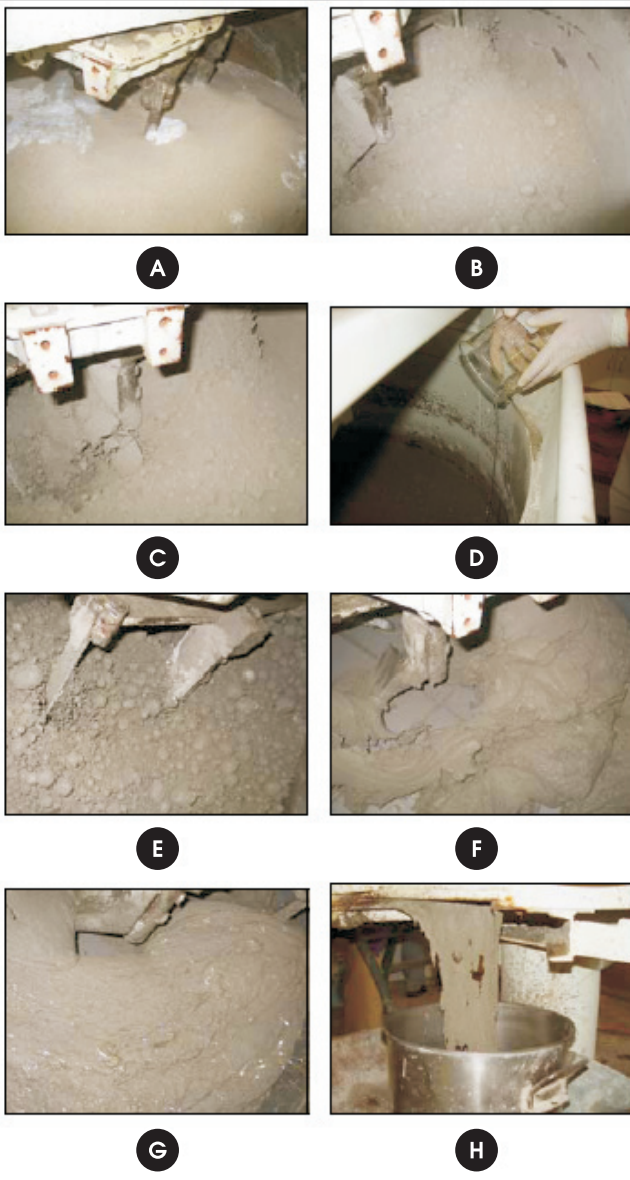
Figure 11 – UHPFRCC mixing steps
